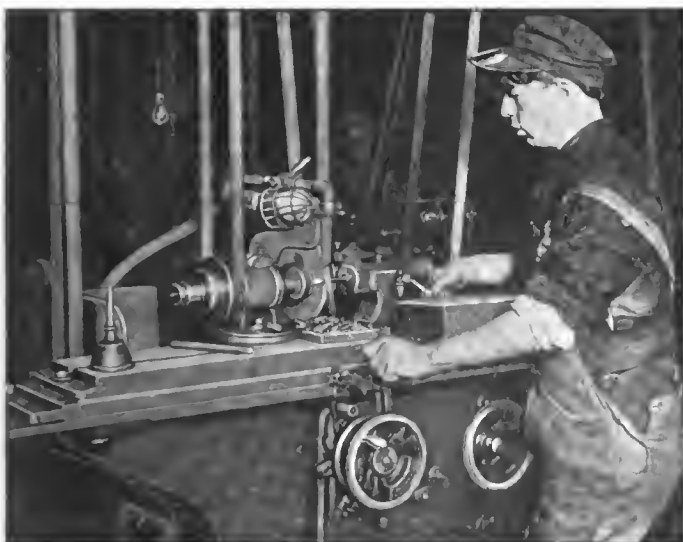
GRINDING TIMKEN TAPER ROLLERS ON AN AUTOMATIC MACHINE.
